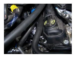
7. AFTER HEADERS ARE IN PLACE. RE-INSTALL FACTORY Y-PIPE ASSEMBLY USING SUPPLIED BOLT KIT. NOW RE-CONNECT BATTERY. CHECK FOR ALL PROPER CLEARANCES THEN START VEHICLE AND THEN CHECK FOR ANY LEAKS. AFTER WARM-UP LET VEHICLE COOL DOWN AND RETORQUE ALL FASTENERS.
